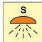
Space protected by sprinkler system 6864 150X150 mm
