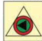
Emergency bilge pump rmt. cont'l 6804 150X150 mm
